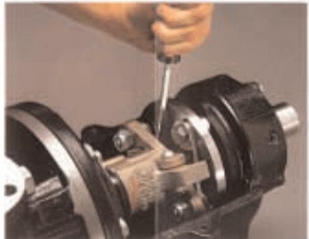
23. Pry the Governor Sleeve forward several times to check for smooth movement and to set the Stationary Seal Ring.
