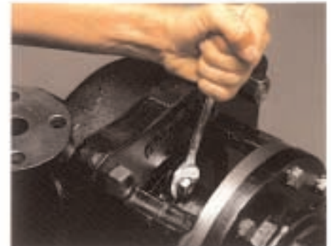
24. Tighten the Stationary Seal Ring Housing Stud Bolt Nuts. Alternate the nut tightening to ensure an even alignment of seals.
