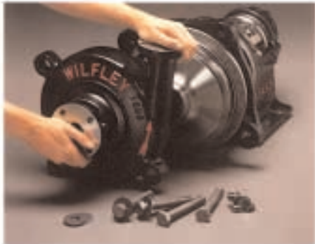
22. Bolt the Case into place.
