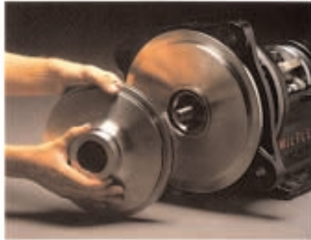
20. Coat threads of the shaft with a non-seizing material and screw on the Impeller.
