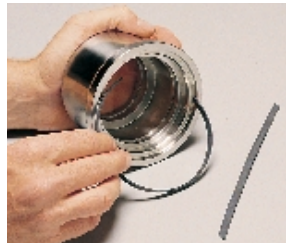
8. Place Slide Rings (24a & b) into bore of Rotary Seal Housing (24). The shorter Slide Ring goes to the rear of the housing. There will be a small gap in the circumference of the seals.
