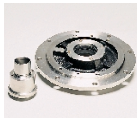
16. Slide the Seal housing assembly onto the Shaft Sleeve Assembly, be careful not to damage the lips of the Stationary Seal during installation.
