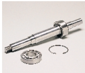
2. Slide Retaining Ring (73) onto shaft, be sure chamfered edge faces away from rear bearing. Install the Inboard Bearing (62a) onto shaft, being sure the bearing groove faces in (stamped side out). Frame 2 requires a cylindrical roller bearing. Install the bearing washer on the shaft prior to the bearing body.
