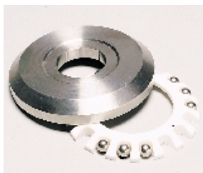
19. Set the Ball Housing on top of the Ball Retainer, be sure the Spring Pin is installed and fits into the hole of the Ball Retainer. Turn the assembly over.
