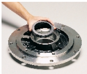
13. Carefully inspect Stationary Seal Ring (23) before installation. The inside surface is the stationary seal face and must be free of scratches or nicks. Insert the seal into the bore of the Seal Housing with the seal face down.
