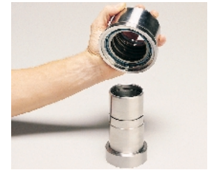
12. Slide Rotary Seal Housing over the Shaft Sleeve. Be careful not to damage the lips of the seal. The Seal Housing (30) must fit completely over the sleeve. Rotate the keyway until it is halfway between the drive screw holes.
