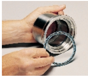
9. Insert the lip seal (25) into the Rotary Seal Housing, be sure the spring faces out. The seal must seat completely in the groove of the housing.
