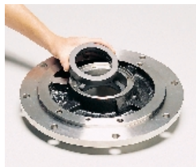
14. Place the Labyrinth Seal or Lube Seal (28) into the bore of the Seal Housing. These seals are symmetrical and can be installed either way.
