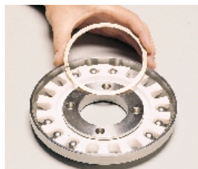
20. Attach the Retaining Ring (34a) to the hub of the Ball Housing.
