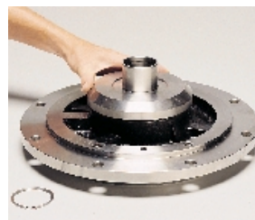
22. Place the Ball housing over the seal assembly, be sure the Drive Screws are seated in the Ball Housing. Press down and compress seal assembly to fit the Retaining Ring (39a) into its groove.
