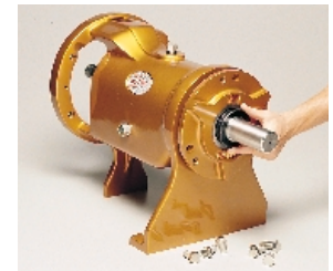
6. Secure the Shaft Assembly to the Frame. Install the Outboard Oil Seal (76) being careful not to damage O-Rings during installation. Some seals have a drain on the bottom. Be sure the seals are installed properly.
