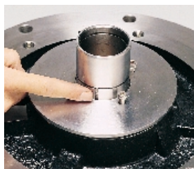
21. Slide the Key (34c) into the slot on the Shaft Sleeve, push down to compress the seal assembly to get the proper fit. A small block placed under the Shaft Sleeve will be necessary to fully compress the assembly. Rotate until the keyway is halfway between two drive screws.
