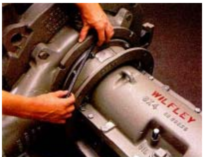
22. Remove the gland ring and install the gland ring packing. Retighten gland ring in place.
