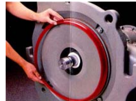
18. Place the follower plate onto the intake chamber and attach the follower plate gasket to the follower plate.
