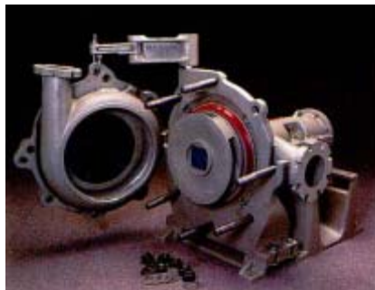
20. Place the case shell gasket on the case shell and attach the case liner to the case shell. Attach the case to the crane arm.
