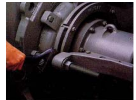
24. Adjust the runner clearances with the draw bolt assembly. Once runner is adjusted properly, securely tighten long cylinder to the frame.
